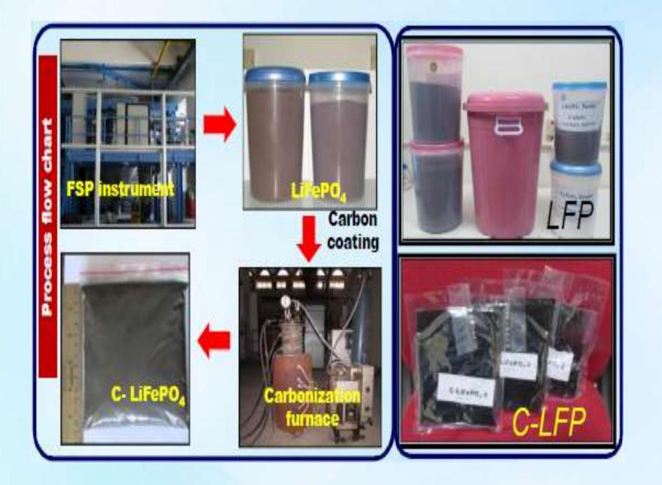
Rs.1700 developed at ARCI. Cost can be reduced by 20% by designing suitable costeffective large capacity furnace and optimum heating cycles with less time
